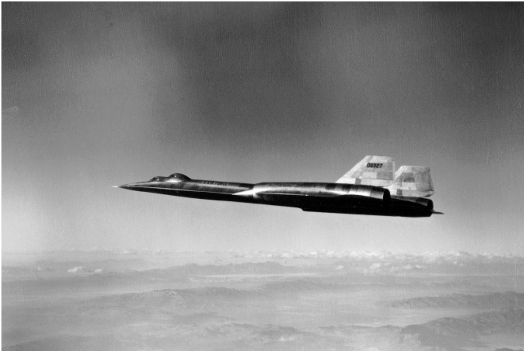
The A-12 trainer during a test flight. Note the two canopies, one for the instructor pilot and another for the trainee. The A-12 trainer aircraft could not reach the upper Mach numbers; CIA pilots experienced that remarkable feat on their own. (CIA)
