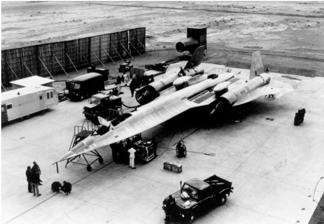
The A-12 Oxcart hidden behind a barrier at Area 51. It took 2,400 Lockheed Skunk Works machinists and mechanics to get a fleet of fifteen ready for the CIA. Visible on either side of the aircraft are the uniquely adjustable inlet cones that regulated airflow and allowed the CIA spy plane to cruise in afterburner and reach peak speeds of Mach 3.29 by May 1965. ( Lockheed Martin )
