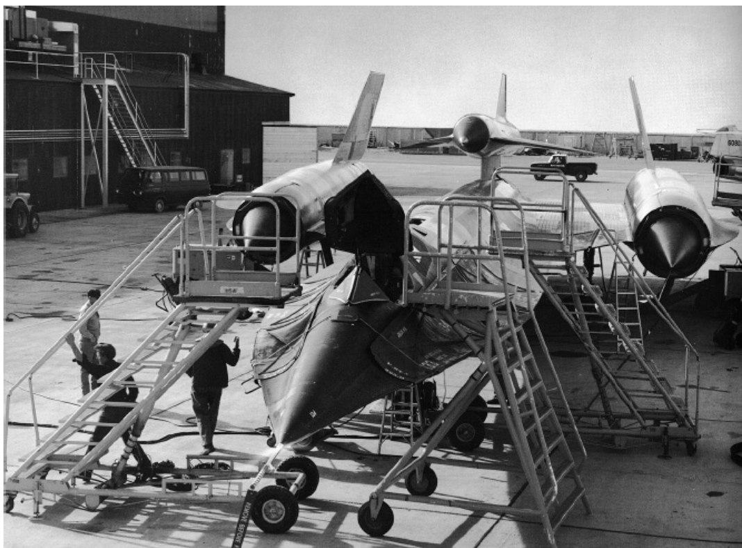
This CIA project, code-named Tagboard, was an Oxcart with a Mach 3 drone on its back, circa 1965. To avoid confusion with the A-12, the mother ship was designated M-21 (as in “mother”) and the drone was designated D-21 (as in “daughter”). ( Collection of Lockheed Martin )
